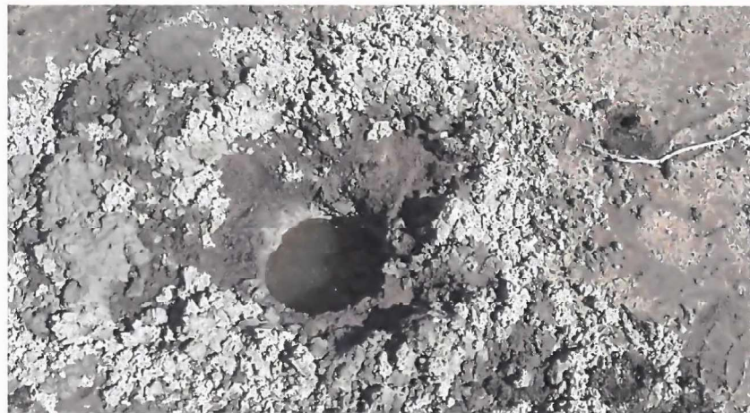
Auger hole in discharge area \approx 2 hours after drilling
